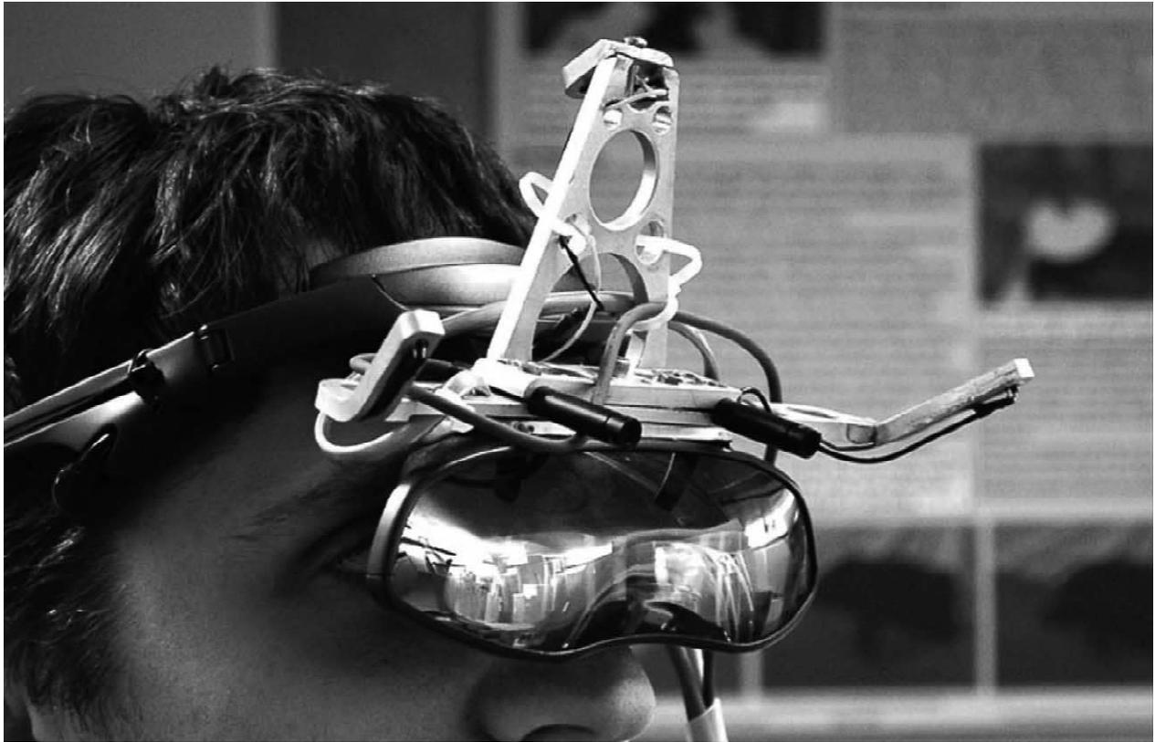
Fig. 3. Video-see-through augmented reality head-mounted display (HMD) built on the basis of a Sony Glasstron LDI-D100 device. The aluminum superstructure holds two miniature video cameras for image capture and three infrared LEDs for opto-electronic tracking of the HMD. A colour version of this figure is available at [www.elsevier.com/locate/media](http://www.elsevier.com/locate/media) (go to Electronic Annexes).
