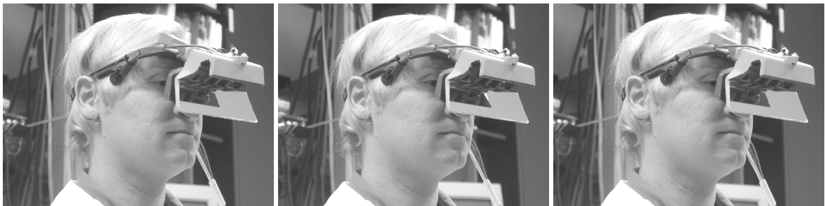
Fig. 4. Ortho-stereoscopic VST-HMD used for the medical AR guidance system. The mirror assembly aligns the miniature video camera to the user's eyes, ensuring continuity between the peripheral field of view and the view through the HMD.
