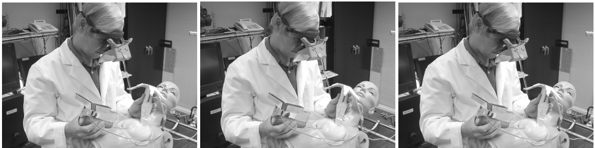
Fig. 1. AR guidance system in use on a breast biopsy training phantom. The user wears a motion-tracked VST-HMD and holds a motion-tracked ultrasound probe (left hand) and a biopsy needle (right hand, also motion-tracked).
