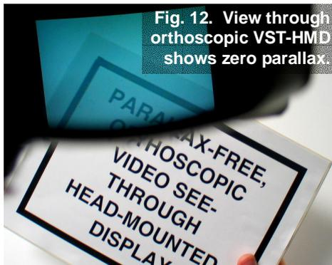
Fig. 12. View through orthoscopic VST-HMD shows zero parallax.
