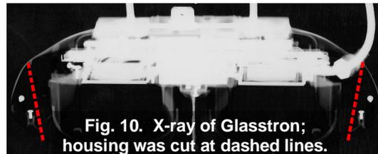
Fig. 10. X-ray of Glasstron; housing was cut at dashed lines.
