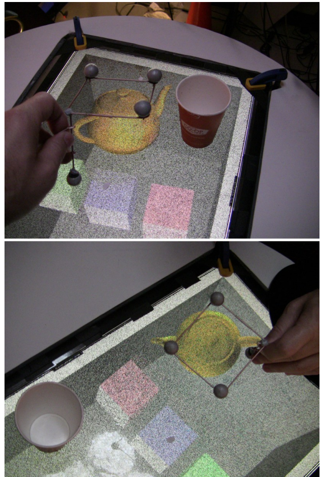
Figure 1: Mixed reality scenario using tabletop autostereoscopic display: Virtual teapot and real cup. The two photos are taken at the same time by two cameras at different positions. Two views are generated simultaneously by the tabletop RHD.
