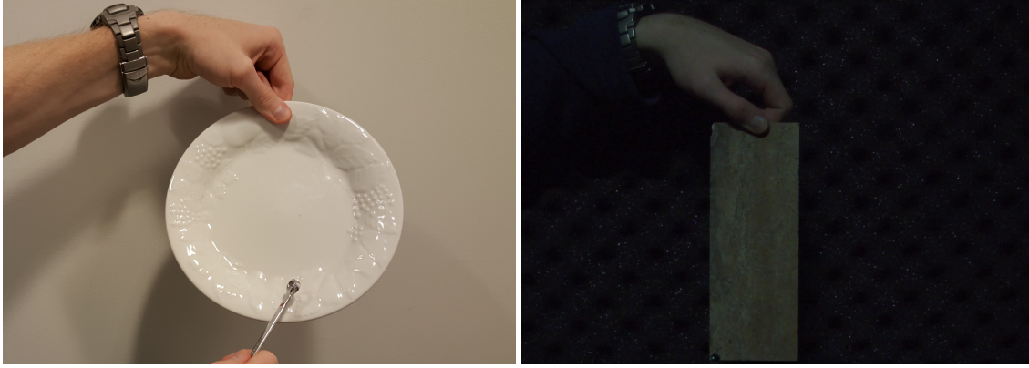
Figure 1.4: A small porcelain plate (left) and a small travertine tile (right) being struck to produce impact sounds. Both objects are supported by a gripping hand. Methods for material damping parameter estimation should be robust to these external damping factors.
