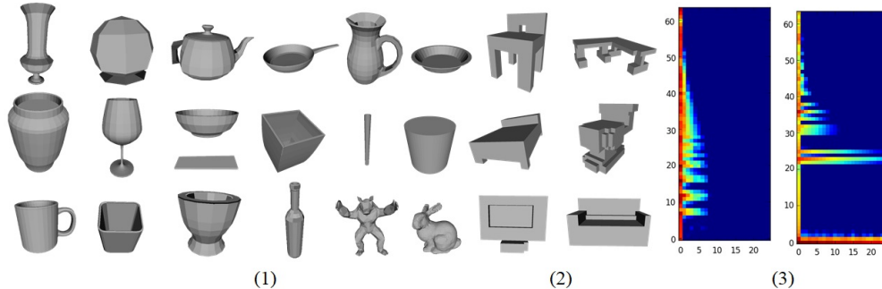
Figure 1.2: We use various datasets for training and testing: (1) our RSAudio dataset with real and synthesized impact sounds from objects of varying shapes and sizes and (2) voxelized ModelNet objects. (3) Audio inputs are formatted as spectrograms.
