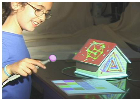
Figure 1. An enthusiastic young user (Miriam Mintzer Fuchs, age 9 years) demonstrates our easy to use system for 3D painting on movable objects. Note that the color palette on the table and the color on the spherical tip of the “paint brush” are projected.
