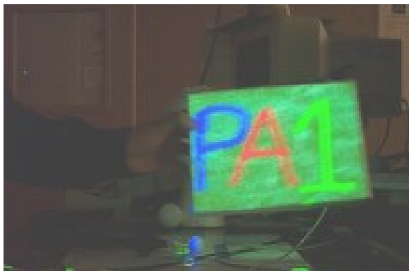
Figure 7. Demonstration of the latency in the tracking pipeline. Notice the blurring and trails artifacts.
