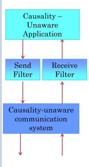
A sent/received message goes through a send/receive filter in send/receive pipeline
