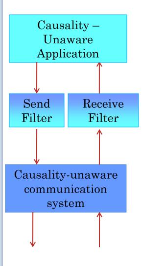
A sent/received message goes through a send/receive filter in send/receive pipeline
