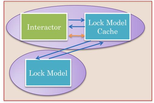
Model cache is a proxy that forwards lock operation without changing its data and forwards release request after changing its data
