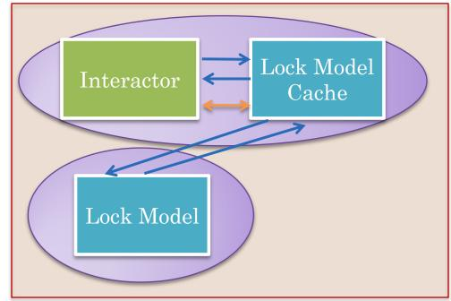
Model cache is a proxy that forwards write (lock, release) operation without changing its data
