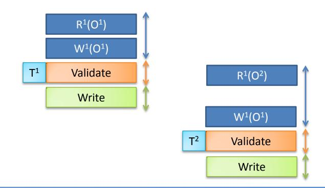
Transaction T<sup>i</sup> is validated if wrt T<sup>j</sup>, j > i, if T<sup>J</sup> does not read any of the items written by T<sup>I</sup> and transaction T<sup>I</sup> finishes its write phase before transaction T<sup>J</sup> begins its write phase.
