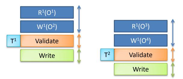
Transaction T<sup>i</sup> is validated wrt T<sup>j</sup>, j > i, T<sup>j</sup> does not read or write any items written by T<sup>i</sup>
