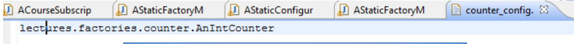
Factory Class reads name of instantiated class from configuration file before factory methods are called
