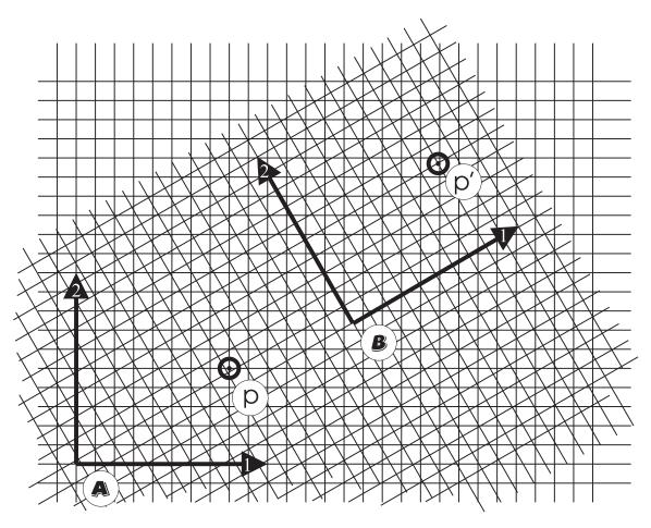
The series of exercises on the following page use this diagram. It shows two coordinate systems, A and B, and two points, p and p'. For your convenience, I have provided a grid aligned with each C.S., which will simplify coordinate measurements. The axis arrows are unit length, so the grid squares have spacing of 0.1 units. Your measurements need not be exact, but take your best guess as to the second decimal place.
