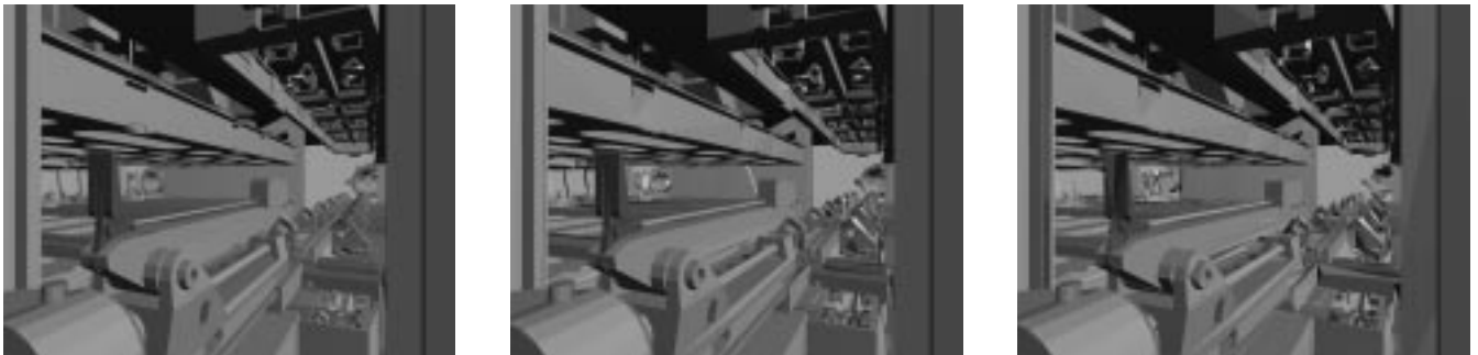
Plate 8: Torp model shown at original resolution (673,728 faces), 0.8% error tolerance (129,446 faces), and 1.5% error tolerance (76,404 faces).
