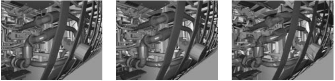
Plate 6: AMR model shown at original resolution (501,550 faces), 0.7% error tolerance (123,106 faces), and 2.5% error tolerance (34,128 faces).
