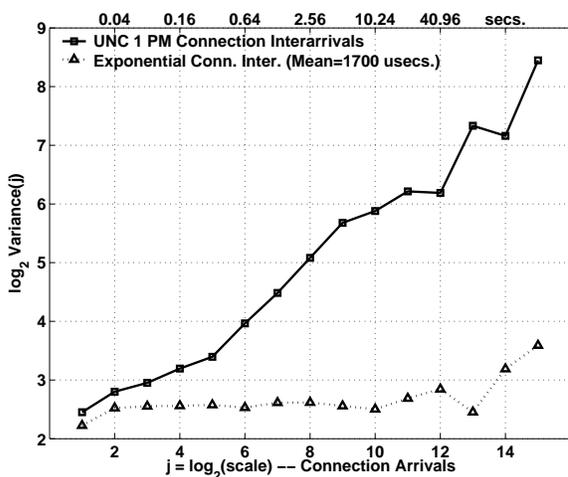
Figure 7.16: Wavelet spectra of the connection arrival time series for UNC 1 PM and a Poisson arrival process with the same mean.
