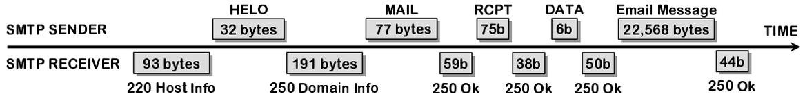
Figure 3.3: An a-b-t diagram illustrating an SMTP connection.
