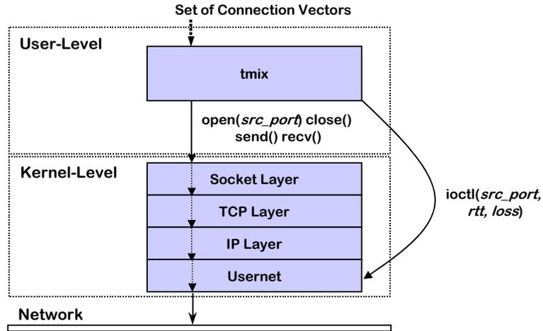
Figure 5.3: End-host architecture of the traffic generation system.
