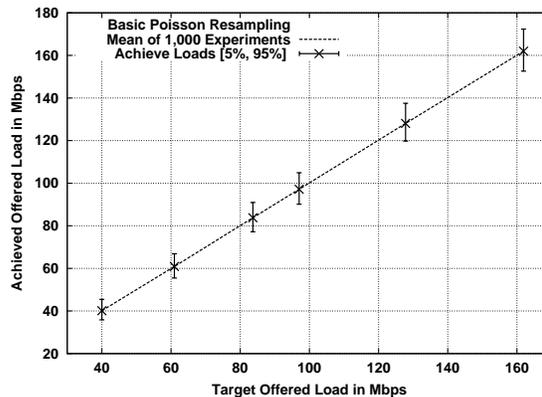
Figure 7.8: Analysis of the accuracy of connection-driven Poisson Resampling from 6,000 resamplings of UNC 1 PM (1,000 for each target offered load).
