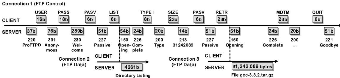
Figure 3.7: Three a-b-t diagrams of connections taking part in the interaction between an FTP client and an FTP server.
