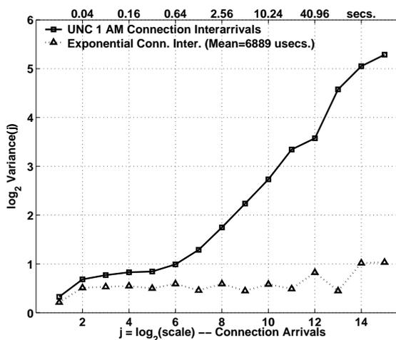
Figure 7.17: Wavelet spectra of the connection arrival time series for UNC 1 AM and a Poisson arrival process with the same mean.
