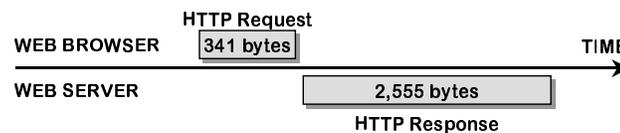
Figure 3.1: An a-b-t diagram representing a typical ADU exchange in HTTP version 1.0.
