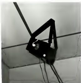
Fig. 1-4a: Detail of fishing-line digitizing unit (from [20])
