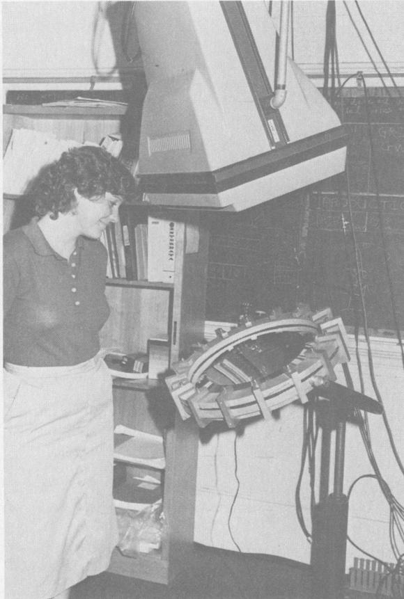
Figure 1. Overall view of UNC display. The CRT is overhead; the mirror is on the stand below.
