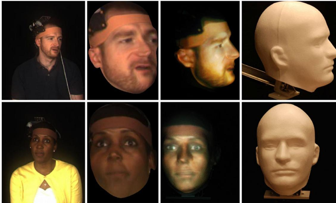
**Fig. 6** Humans and Avatars as seen from different viewpoints. *Column 1* shows the live camera images; *column 2* shows the warped head models; *column 3* shows photographs of the models projected onto the Avatar; *column 4* shows the un-illuminated styrofoam head
