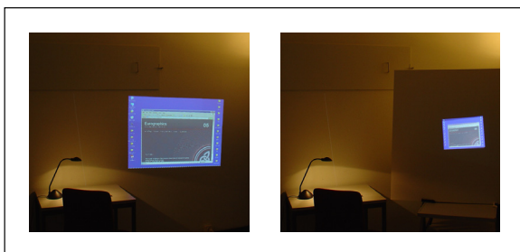
Figure 20: Instant displays can be redefined with a laser pointer, allowing a user to move projections to new surfaces.
