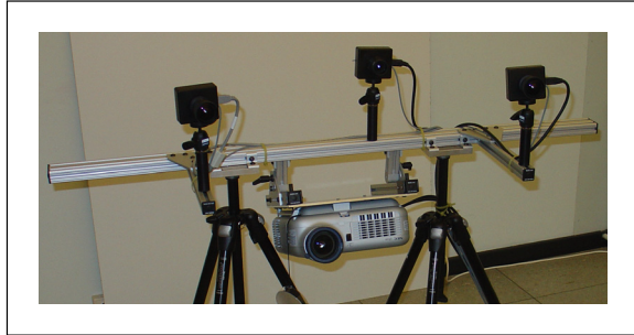
Figure 2: Instant display brick with projector and cameras.
