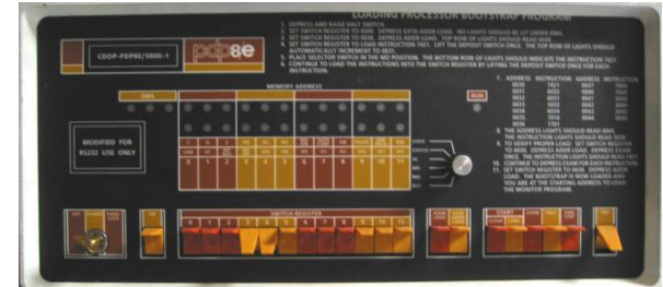
Front panel of a classic PDP8e. The toggle switches were used to enter machine language.
