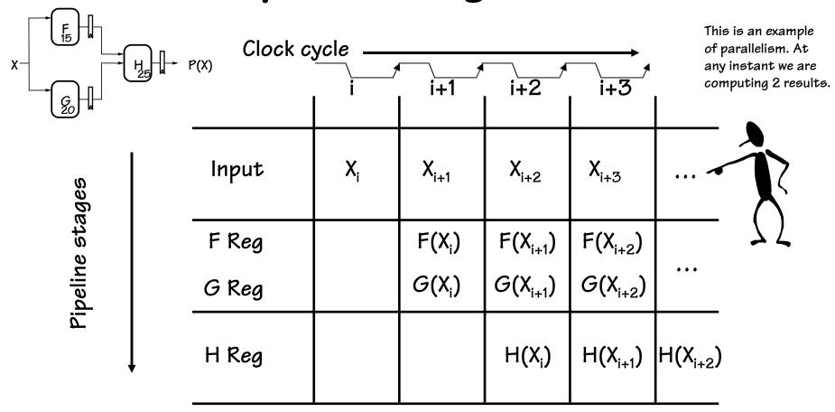
The results associated with a particular set of input data moves diagonally through the diagram, progressing through one pipeline stage each clock cycle.
