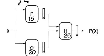
Now F & G can be working on input  $X_{i+1}$  while H is performing its computation on  $X_i$ . We've created a 2-stage pipeline: if we have a valid input X during clock cycle j, P(X) is valid during clock j+2.
