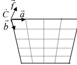
Figure 2. Parallel projection camera representation.
