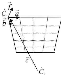
Figure 4. Parallel and perspective projection cameras that share the same image plane (origin,  $\bar{a}$  and  $\bar{b}$  vectors).
