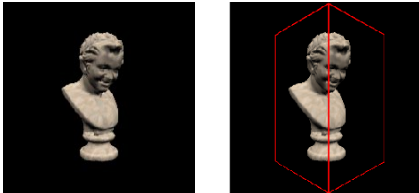
Figure 16. Reconstructed view of the statue obtained by texture mapping two quads (left). The red lines show the boundaries of the polygons (right).
