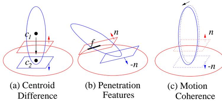
Figure 5: Various Initial Guessing Strategies. (a) shows that the centroid difference vector  $c_2 - c_1$  can approximate the penetration direction. (b) shows that the normal vector  $n$  of a penetration feature  $f$  approximates the penetration direction. (c) shows that the PD computation result (penetration vector  $n$ ) from the previous time frame can provide the penetration direction.
