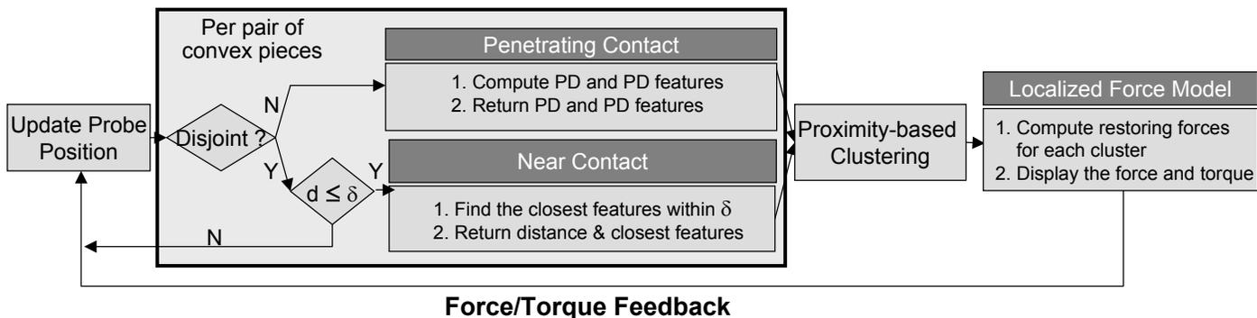
Figure 1: Haptic Display Pipeline
