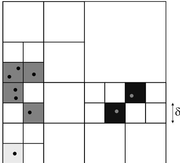
Figure 2: Contact Clustering Using Quadrees. *The contacts are represented by dots. Different intensities are used to highlight the different clusters. Octrees are used instead of quadtrees in our 3D implementation.*
