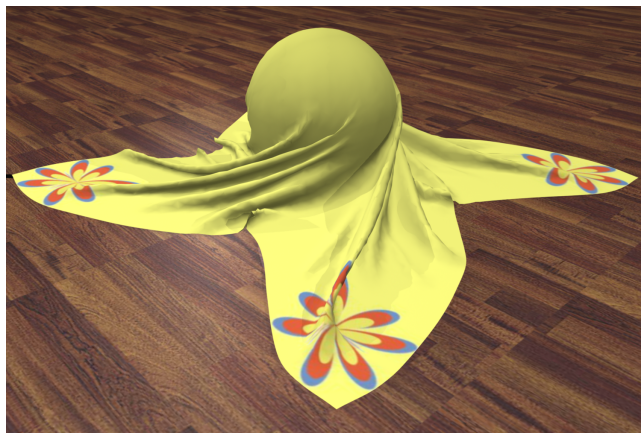
Figure 2: Cloth simulation: The cloth mesh is composed of 15K triangles and has a high number of triangles in close proximity. As the simulation progresses, the cloth wraps around the sphere and the simulation generates many complex folds. Our algorithm is able to perform continuous self-collision detection among all the triangles within 800 msec.
