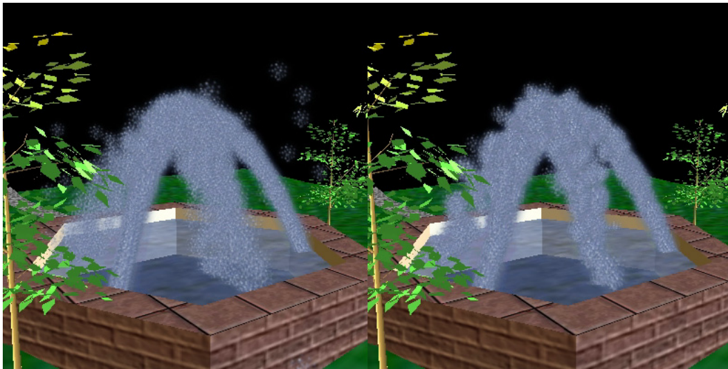
Figure 9. Two snapshots of the fountain simulation. The left simulation uses no SLODs, while the right one uses SLODs with a maximum cluster size no greater than 30. The SLOD simulation runs 6 times as fast and maintains a consistent frame rate.
