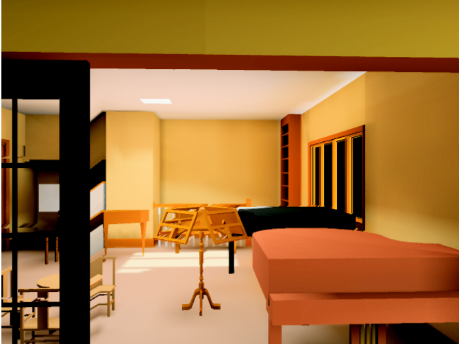
Plate 3: A particularly bad derived frame produced by our test-bed. Some areas of the image near the door were occluded in both reference frames, mostly because of prediction error. Low-connectedness triangles, which are colored using our heuristic technique, are visible in these areas. This frame is from the same sequence as Plate 1.
