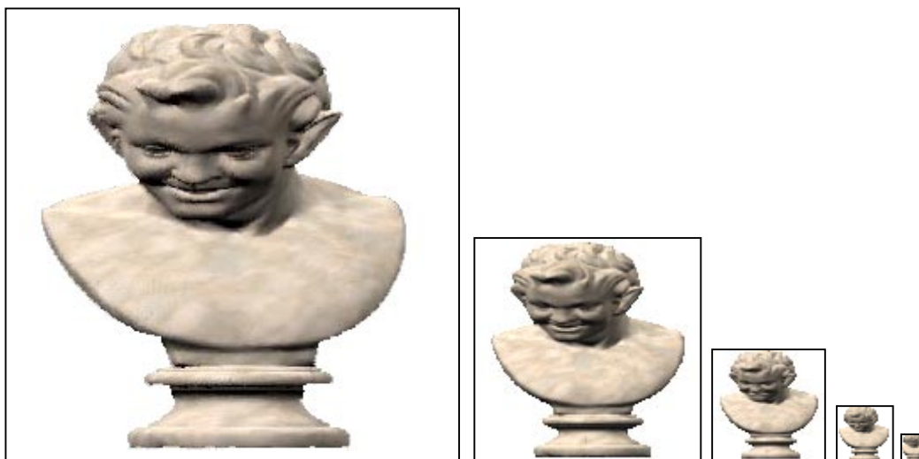
Figure 6-1. Relief texture pyramid showing five levels for the front face of the statue. From left to right the dimensions of the textures are respectively 256x256, 128x128, 64x64, 32x32 and 16x16 texels.
