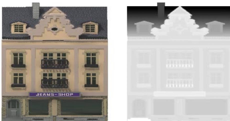
Figure 3-27. Actual 256 by 256-texel color image and depth map used to create illustrations for this chapter.
