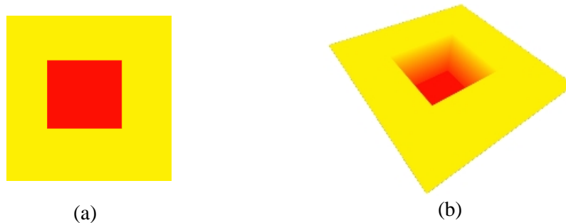
Figure 4-29. Sharp depth discontinuities matched by color change. (a) Source image used in conjunction with the depth map shown in Figure 4-10. (b) Oblique view of the resulting surface rendered with a two-pass 1-D warping and resampling algorithm. The results obtained with both orders ( i.e. , horizontal and vertical first) are similar to a 2-D resampling.
