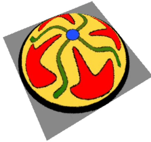
Figure 2-15. Perspective view of the texture-mapped surface obtained after applying the texture shown in Figure 2-14 (left) to the surface shown to its right.
