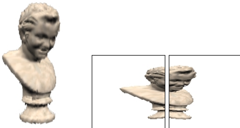
Figure 6-3. Textured LOD produced with 128x128-texel relief textures. The corresponding pre-warped textures are shown on the right.
