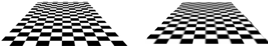
Figure 6-6. Checkerboard texture mapped using bilinear (left) and trilinear (mip mapped) resampling (right).
