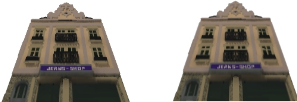
Figure 6-8. Building façade pre-warped and then texture mapped using bilinear (left) and trilinear (mip mapping) resampling (right).
