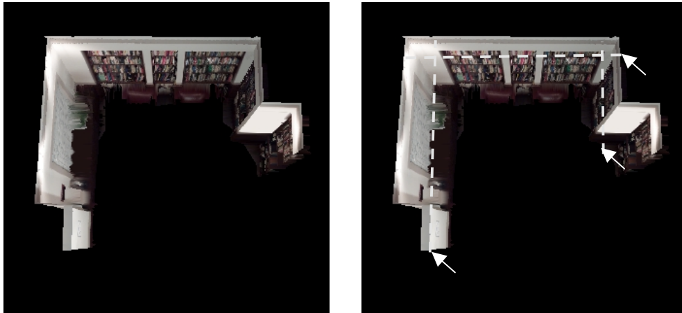
Figure 5-23. Sitterson Hall’s reading room (partial model seen from above). Spatial relationship among the walls (left). Dashed lines represent the planes used for relief texture acquisition (right).
