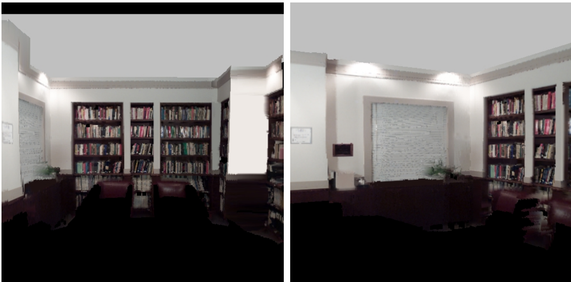
Figure 5-26. Room rendered using relief texture mapping. Notice the parallax effect that allows the plaque to become visible in the image to the right.
