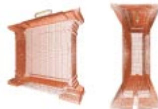
Plate 6 (Figure 17). Close-ups of the old clock rendered as point clouds to illustrate back face culling (front and opposite side culled).
