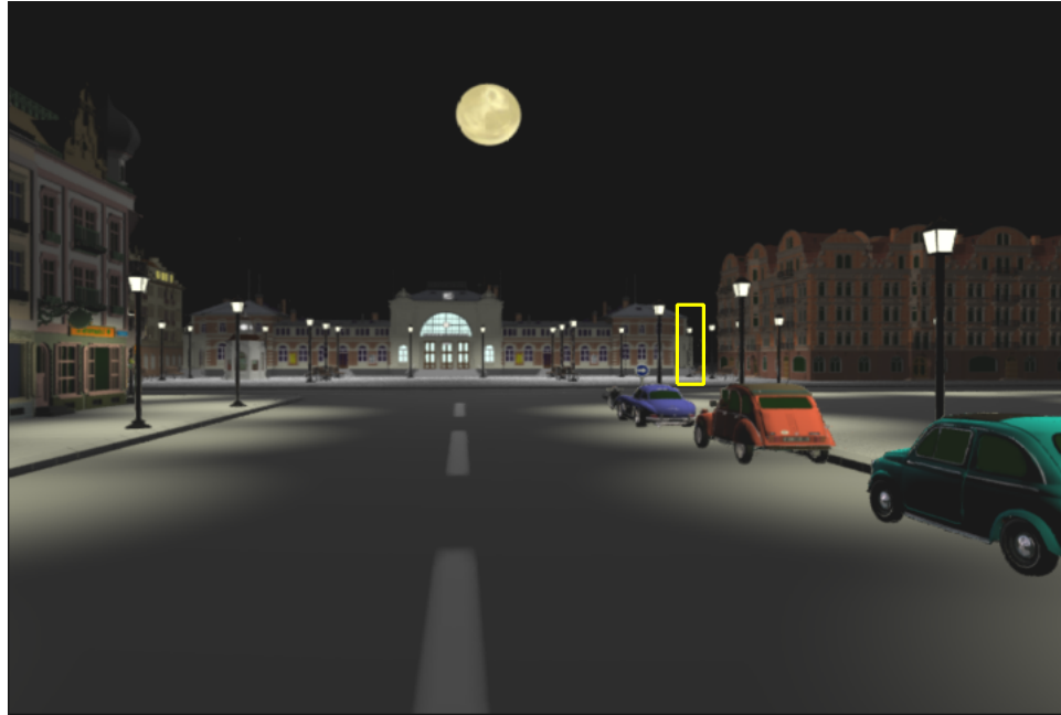
Figure 4.5. Elimination of thin features as edge samples are discarded. The artifact is well illustrated by some of the light poles in the distance, like the one in the box.
