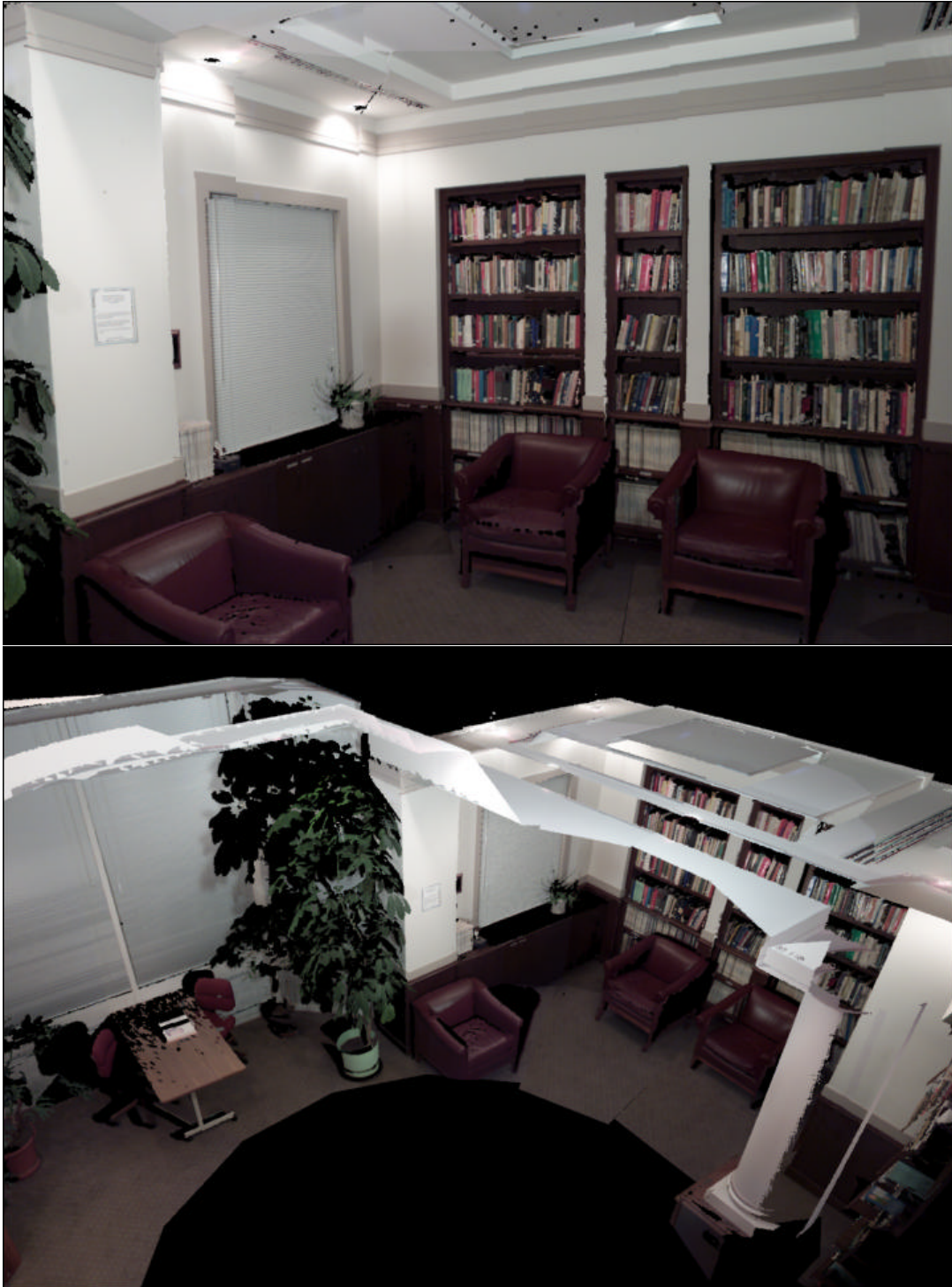
Figure 1.7 Rendering method tested on a natural scene. The reference depth-images of the reading room were created by registering color images with the range information acquired by our in-house laser rangefinder. The rangefinder captured data from two positions in the center of the room. We are missing some data, on the ceiling for example, but the surfaces for which data was available are rendered realistically.
