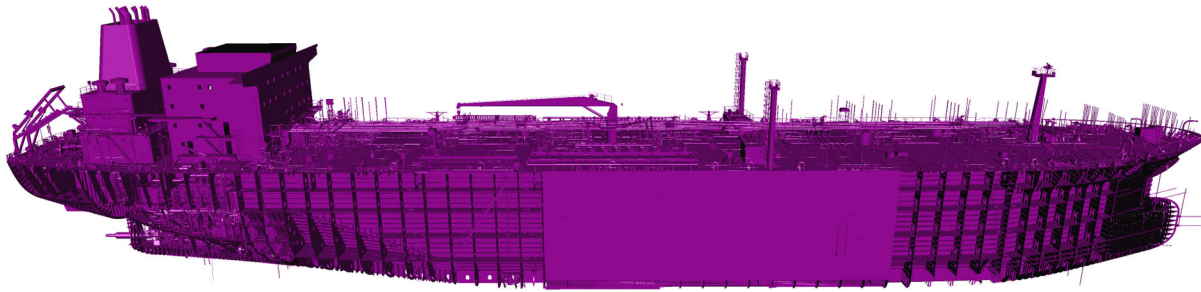
Figure 7.2: Less than 1 MB of memory is used by the out-of-core process that loads, decompresses, and renders this 82 million triangle “Double Eagle” model in 78 seconds from a 180 MB file. We do not store triangles in memory, but immediately render them with one call to glNormal3fv() and three calls to glVertex3iv() . Loading and decompression alone takes only 63 seconds. Most of the additional 15 seconds are spent on computing triangle normals. This frame was captured in anti-aliased 2048x768 dual-monitor mode on a 1.8 Ghz AMD Athlon processor with an Nvidia Geforce 4200.
