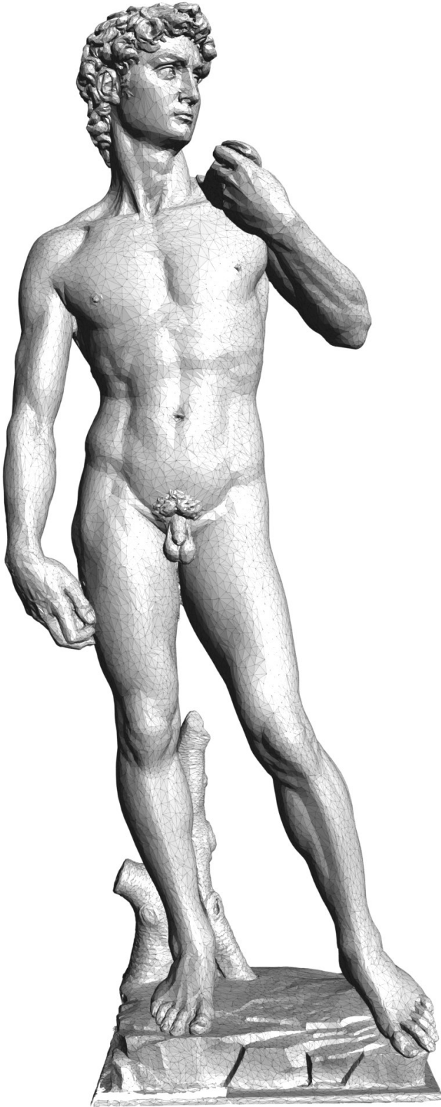
Figure 8.9: Adaptive simplification of David (2mm) to 1% of the input mesh with a stream-based simplifier using processing sequences and buffer-based processing.
