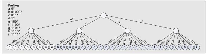
■ Figure 16. A two-level fully expanded multibit trie.
