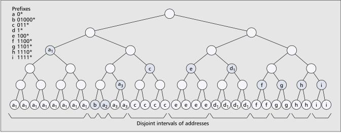
■ Figure 11. An expanded disjoint-prefix binary trie.
