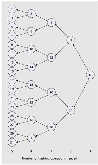
■ Figure 23. Standard binary search on lengths for IPv4.
