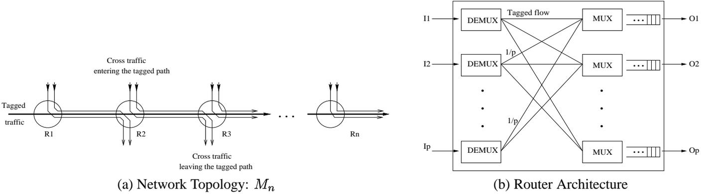
**Figure 2:** Simulation environment: network topology and router architecture
