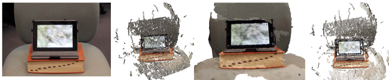
Fig. 10. From left to right: sample dataset imagery, respective outputs of PMVS, CPMVS and our proposed method.
