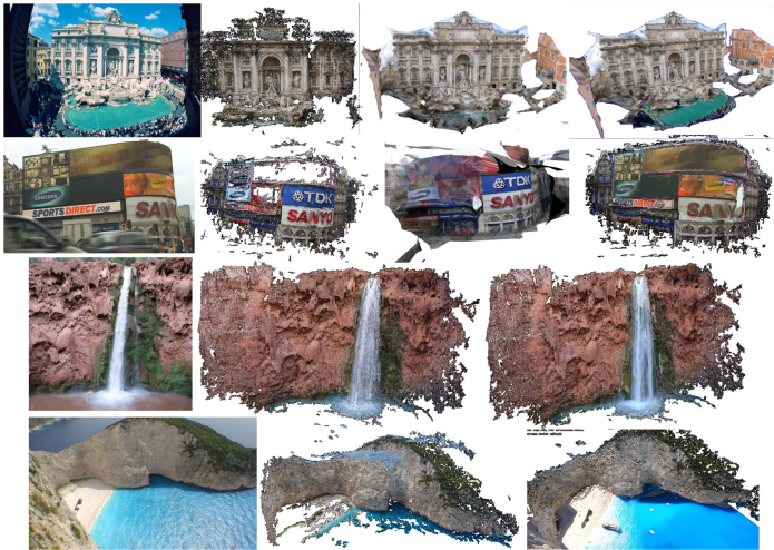
Fig. 9. Top two rows: sample dataset imagery, respective outputs for PMVS, CPMVS and our proposal. Bottom two rows: sample dataset imagery, respective outputs for PMVS and our proposal; CPMVS failed to generate on the same input data.
