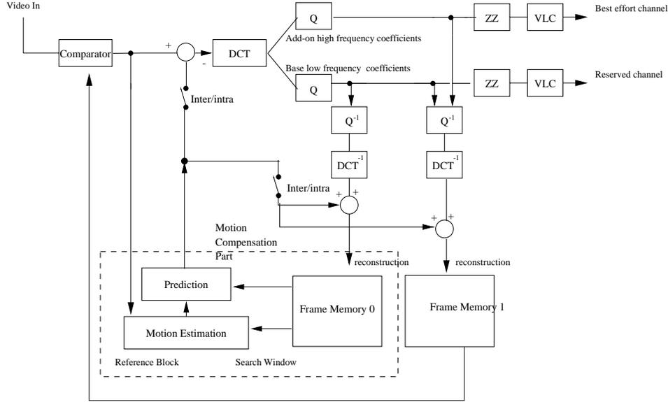
Figure 2: Reservation-based video coding scheme.
