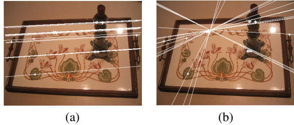
Figure 3. (a) Correct epipolar geometry computed by QDEGSAC valid for all points. (b) Epipolar geometry computed by RANSAC only valid for points on the tray (plane).
