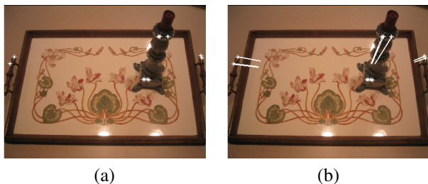
Figure 8. (a) reprojection error for the projection matrix estimated with QDEGSAC (b) reprojection error of a RANSAC solution.
