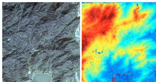
Figure 1. Left: Stereo disparity for high resolution satellite images (150M) is a computationally intensive task evaluating upwards of 1000 hypotheses per pixel. Right: Output from our proposed SOS<sup>+</sup> framework, space reduction enables an order of magnitude reduction in computational complexity.
