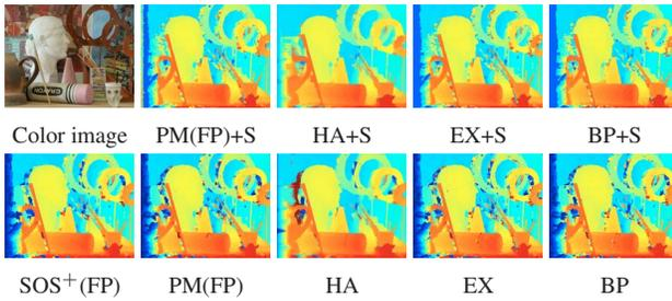
Figure 7. Raw disparity maps for various stereo methods.
