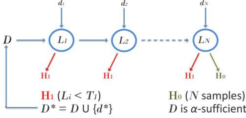
Figure 3. Sequential Optimal Sampling (SOS) model. Given a depth set  $D$  and a new observations  $d_i$ , if the accumulated likelihood drops below threshold  $T_1$ ,  $D$  is augmented. Sampling halts after  $N$  consecutive samples without updates to  $D$ .
