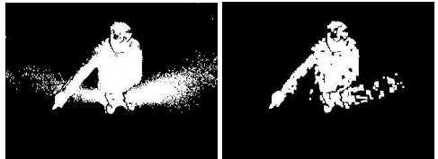
Figure 4: segmented image with the applied threshold (left) and image with removed shadow based on NCC (right)
