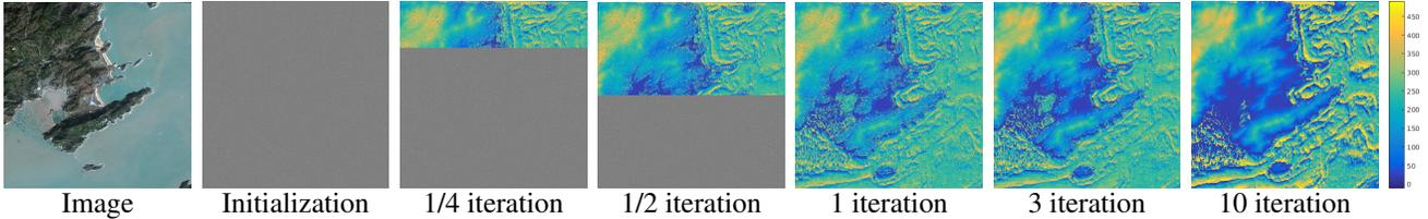
Figure 3. Qualitative illustration of convergence. We show the height map obtained at different stages of the optimization process. The first iteration already extracted coarse geometrical structures from the random initializations. Results obtained after 3 iterations are visually very close to the final results with 10 iterations.
