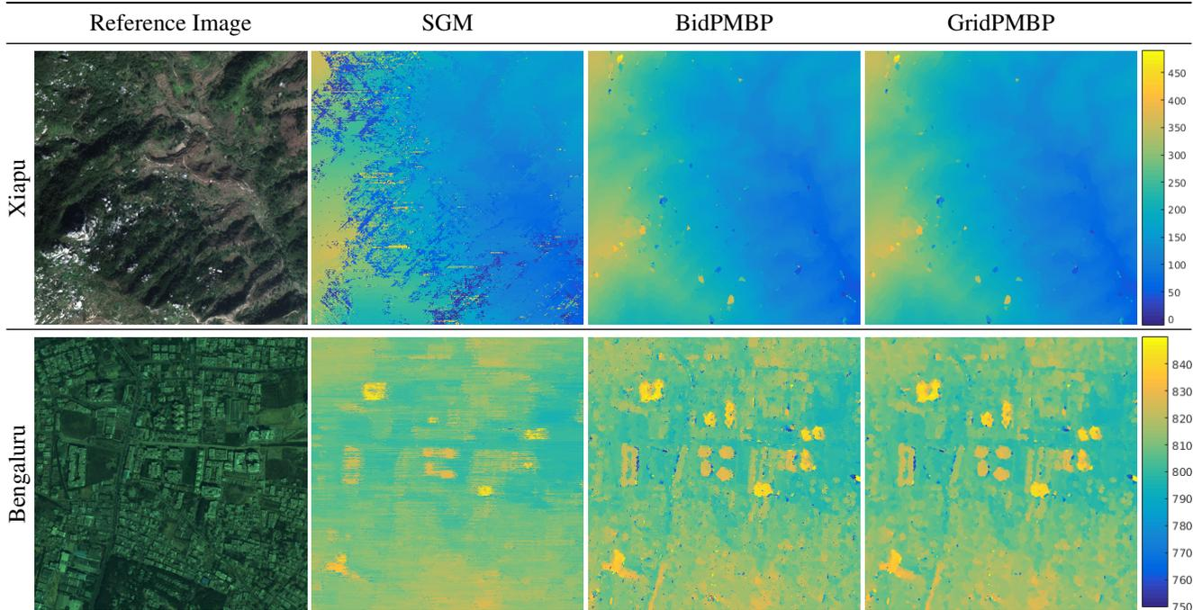
Figure 8. Zoom in comparisons of satellite height map estimation results. GridPMBP provides cleaner results with much smaller computation and memory overhead. (Best view in color.)
