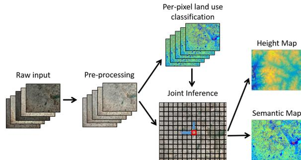
Figure 1. Schematic description of our pipeline. Pixel values of the given set of satellite images are first converted from native radiance to top-of-atmosphere reflectance. Land usage labels and converted images are used together in the MRF inference process to get refined geometric and semantic estimates.
