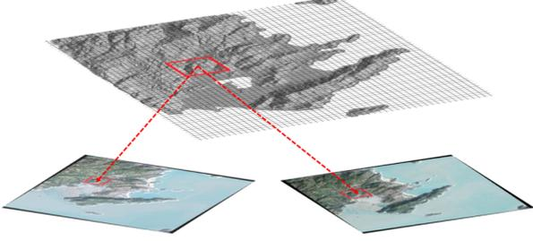
Figure 2. Visualization of the grid representation of our proposed method. Each grid point is parameterized by a local 3D plane and land usage information. Photo consistencies are accumulated across multiple images.
