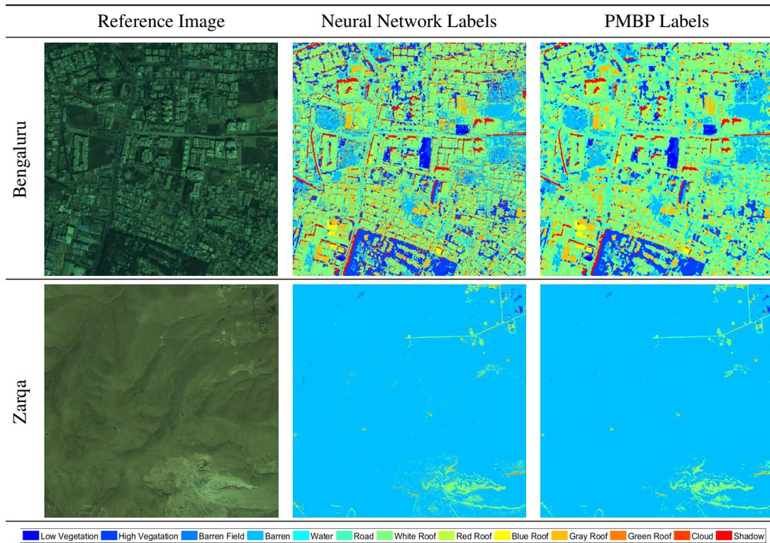
Figure 7. Comparison of semantic labels. Per-pixel based classification can lead to noisy semantic labels, see column 2. By joining dense stereo estimation together with per-pixel classifications, noisy semantic maps can be smoothed, see column 3. (Best view in color.)
