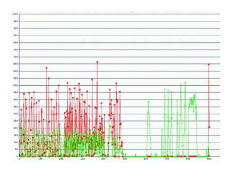
**Fig. 5.** Bandwidth usage plot from Nov 19 2002 SuperComputing 2002 demonstration, showing Mbps over time. The darker line (red) shows the data traffic from acquisition to computation site, while the lighter line )green) shows the traffic from computation to display site.
