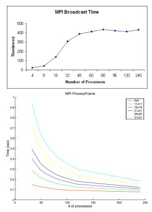
**Fig. 4.** Left: The time required to broadcast images to each node increases as the number of processors increases. Right: Total processing time in msec vs number of processors. Each plot corresponds to a different kernel size.
