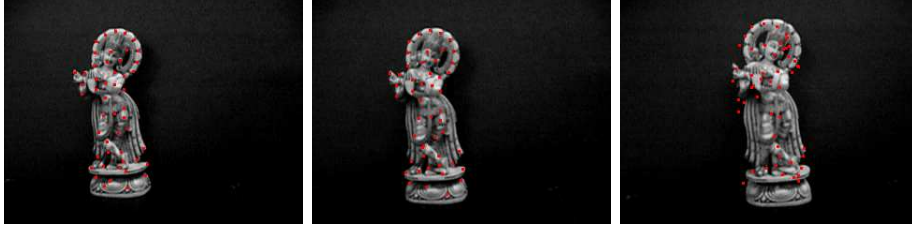
Figure 2: Features tracked by the HRBF-augmented KLT tracker.
