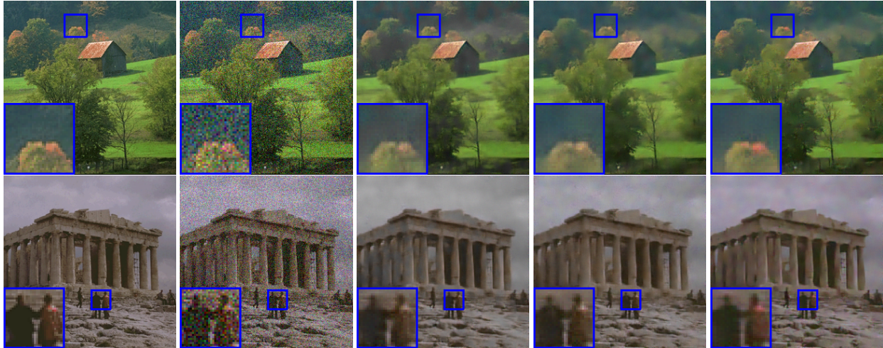
Fig. 3. Columns from left to right: Original image, the image with noise of \sigma = 25 , K-SVD denoising result [5], improved K-SVD denoising result [8], our K-QSVD denoising result.
