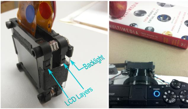
Figure 11: Prototype hardware and testing configuration. *Left*: Prototype display unit for one eye, consisting of two stacked LCD microdisplays and an RGB backlight. *Right*: Testing configuration for experiments described in Section 5.2. The camera setup was configured to approximate a human wearing eyeglasses: the camera lens was placed nearly in contact with the display so that the display to camera center of projection distance was 18 mm, and a 3.7 mm aperture was used.
