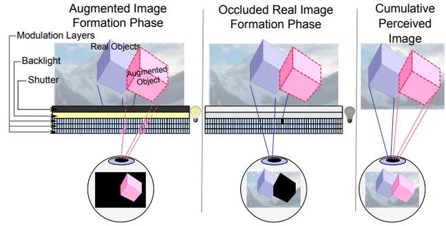
Figure 3: Method of operation. *Left*: In the first phase, an augmented image is formed through the backlight and spatial light modulation layers while the real scene is blocked by the shutter. *Center*: In the second phase, an occluded real image is formed by opening the shutter and blocking light rays from real objects that coincide with augmented objects. *Right*: The two phases alternated in rapid sequence form a perceived AR scene with opaque augmented objects.
