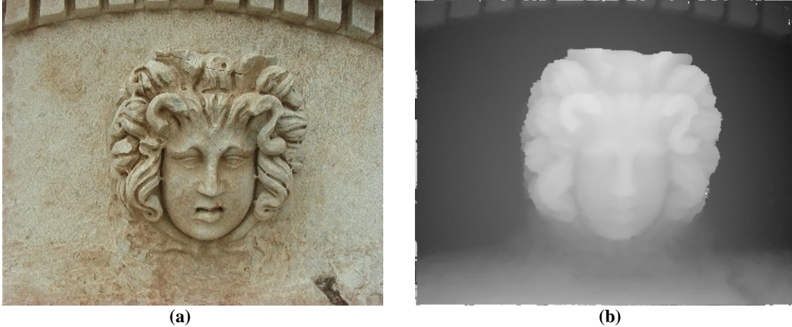
Figure 4: a) Image extracted from a video and b) computed depth map.
