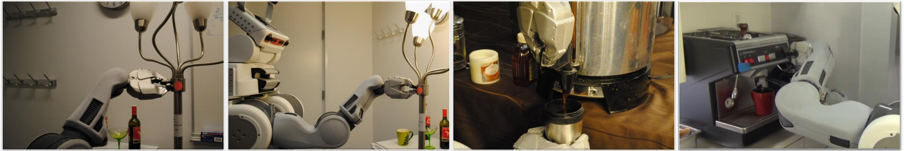
Fig. 10. Examples of transferred trajectories being executed on PR2. On the left, PR2 is able to rotate the ‘knob’ to turn the lamp on. In the third snapshot, using two transferred trajectories, PR2 is able to hold the cup below the ‘nozzle’ and press the ‘lever’ of ‘coffee dispenser’. In the last example, PR2 is frothing milk by pulling down on the lever, and is able to prepare a cup of latte with many transferred trajectories.
