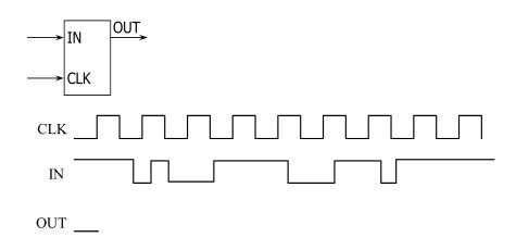
15. (3 points) Refer to the following circuit. Suppose the propagation delay of each flipflop is 1 ns (i.e., the delay from the up-transition of the clock to the data appearing at the flipflop's output), and suppose that the setup time for each flipflop is also 1 ns, and the hold time is zero.
