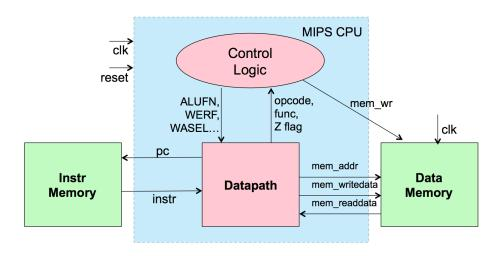
Small amounts of logic can be "inlined" (instead of written as a separate module), e.g., muxes, sign extension, adders, shift-by-2, etc.
