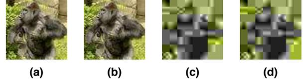
Fig. 2. A  $64 \times 64$  resolution image compressed in high/low quality settings using JPEG/JPEG2000: (a) JPEG high quality, 1963 bytes (b) JPEG2000 high quality, 2026 bytes (c) JPEG lowest possible quality, 738 bytes (d) JPEG2000 lowest possible quality, 391 bytes.
