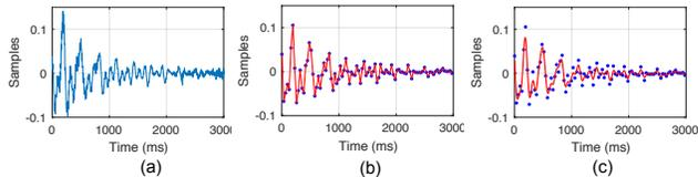
Figure 9: Predicting missing values of signal(a) using linear(b) and spline(c) interpolation.
