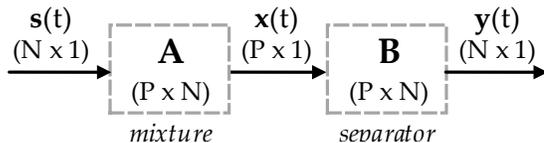
Figure 1: Generic model for source separation.
