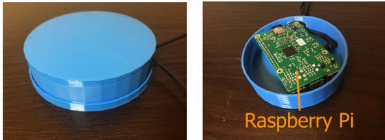
Figure 11: Alexa-enabled Raspberry Pi in a case.
