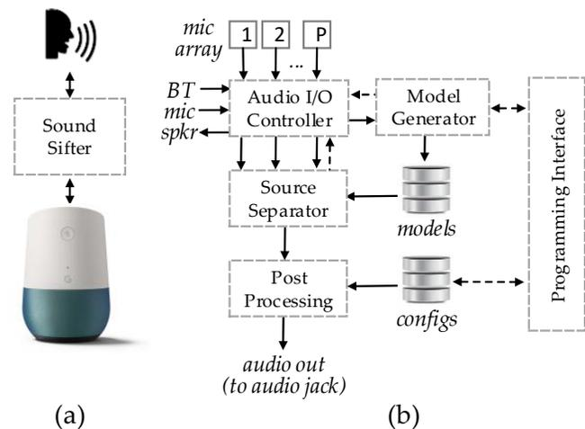
Figure 2: (a) System interface, and (b) block diagram of SoundSifter.
