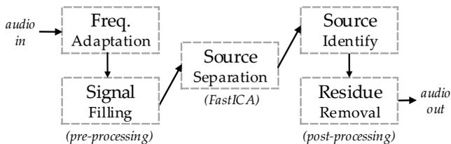
Figure 7: Components and interconnections inside SoundSifter’s audio processing pipeline.
