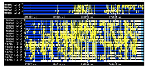
Fig. 5. PARAVER time charts for T3 on 4 vs. 16 processors of OSC's P4 cluster
