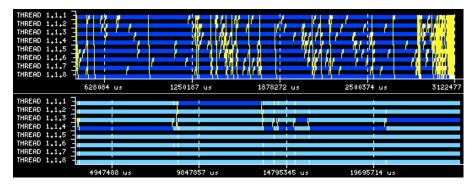
**Fig. 9.** PARAVER time charts for T1 exploration at chunk sizes of 10 nodes (top) and 60 nodes (bottom) on the Origin 2000
