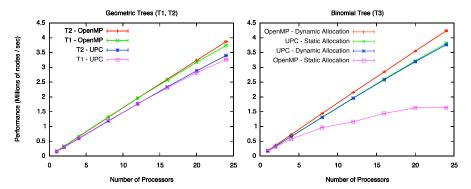
**Fig. 3.** Parallel performance on the Origin 2000 using OpenMP and UPC. On the left, results for geometric trees T1 and T2. On the right, results for T3 with static versus dynamic data allocation for the steals stacks. Optimal chunk sizes were used.
